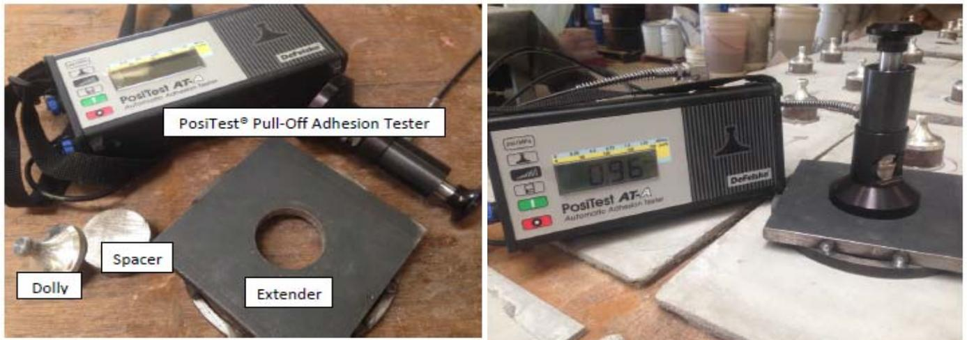
Figure 2 – Pull test apparatus and set-up.
