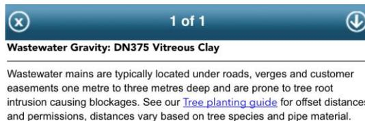
Pipe sizes are displayed in "Diameter Nominal" format (eg. DN300). The number after "DN" is the diameter of the pipe, measured in millimetres.
